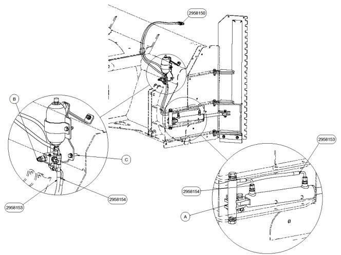
A: The bracket for the cylinder must be installed as in the illustration.
